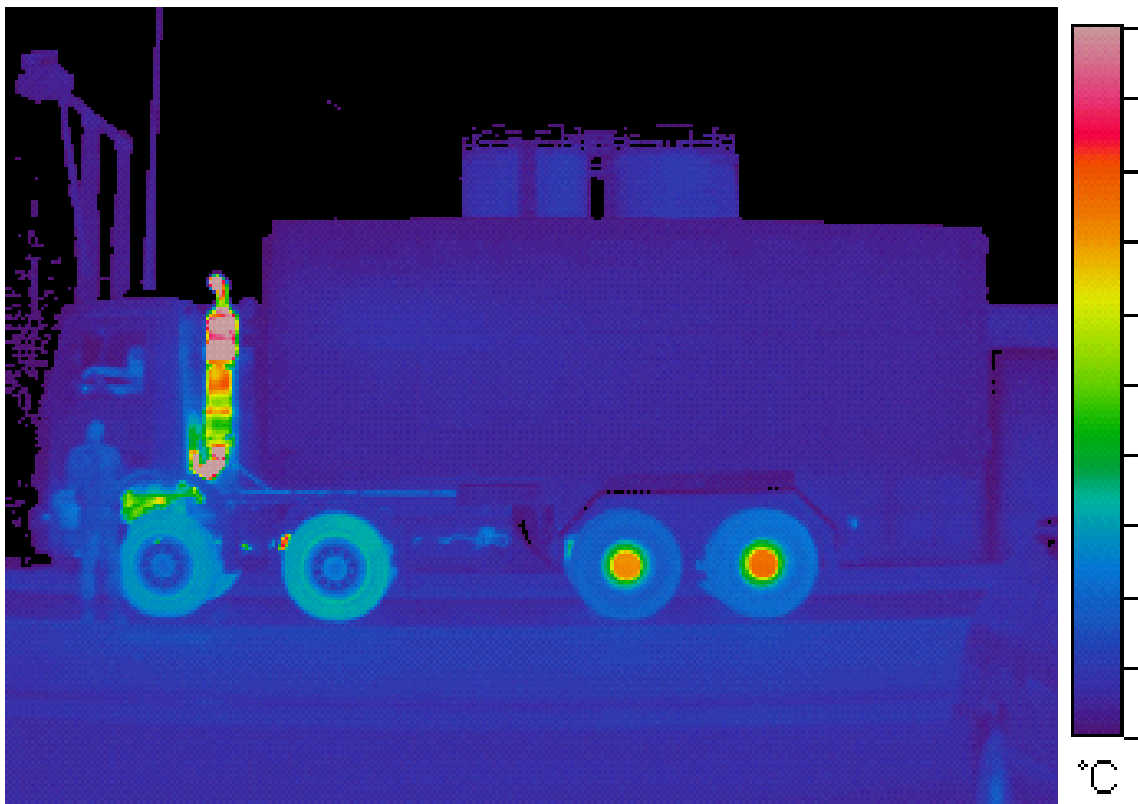
Diverted vehicle: view of exhaust system and turbo charger. Both rear axels are visibly warmer (braking energy)
